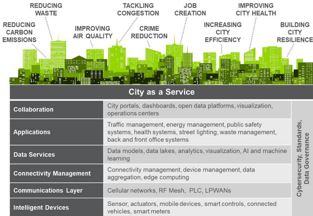
Figure 4-1. The Smart City Platform
