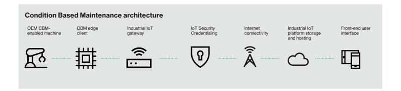
CBM, which is delivered as a service on our Asset Tracking and Management IoT platform, transforms physical assets into virtualized, software-based models with integrated analytic fields. Third-party sensors are connected to the equipment and, using IoT Security Credentialing architecture, securely relay diagnostic data to the Condition Based Maintenance platform, so you get the insights you need to keep your equipment up and running smoothly.
