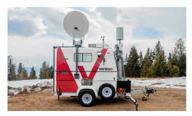
A Mobile Connectivity Trailer enables rapid creation of a cellular coverage area.
